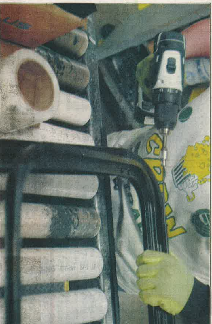
J. Tyler Klassen/The Elkhart Truth Chrystal Leighton screws a set screw into a window at State Wide Windows in Elkhart on Thursday, June 26. Leighton has been with the company two years.
