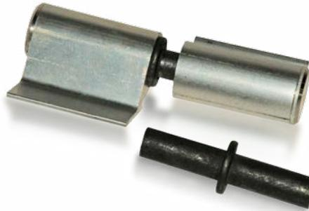
*A mill extrusion with a longer flange, graphite pins and heavy-duty components are evident at first glance on the Clydesdale Series. Stronger hinges are welded to the frame rather than riveted.*
